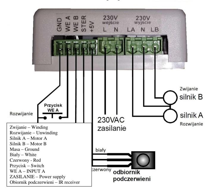
Start installation of the module by wiring the motor of the screen/lift drive to the module. Proceed with wiring the motor connections in the following sequence:
