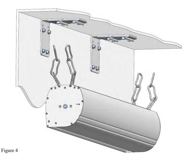
5. The bracket mounting system is shown in the figures below. Fitment of the screen can be described in three steps
