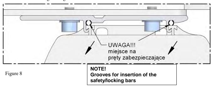
6. Lock the suspended screen housing using the safety/locking bars by sliding them in the groove between the bracket and the housing. Figures 8, 9a and 9b show the insertion sequence and location.
