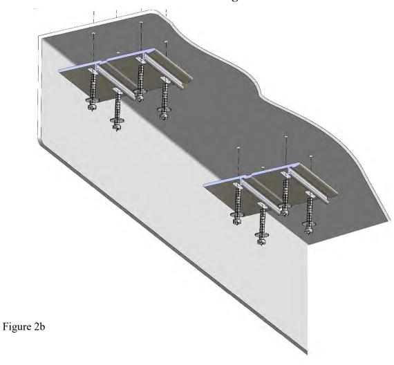
3. In case of wall installation, assemble the flat and angle brackets using the screws supplied in the installation kit.
